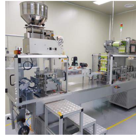
PTP packaging machine (60,000 packs/8H)
