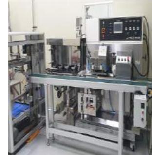
10 row stick packing machine(810,000 bags/ 8H)
