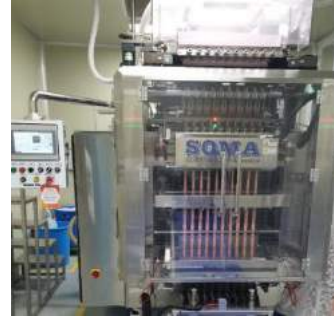
10 row stick packing machine(810,000 bags/ 8H)
